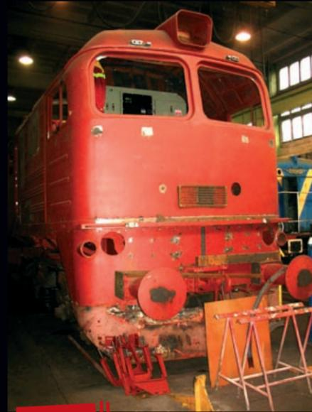
**TOTALLY REBUILT** and remanufactured carbody from standard M62 locomotive
