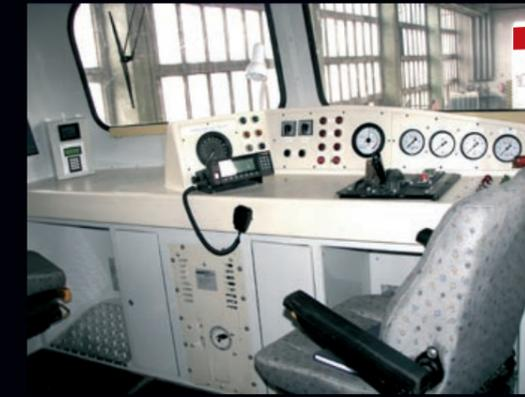
**ERGONOMICALLY DESIGNED** drivers cabs with simple and functional control layout
