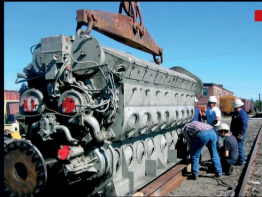
**RELIABLE AND FUEL** efficient 16 cylinder, 2238 kW, EMD model 645E3C diesel engine
