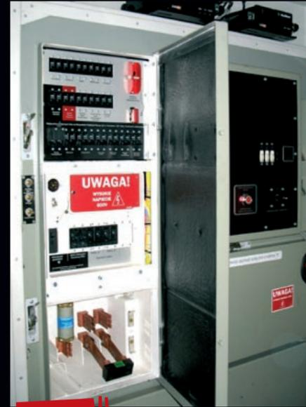
**SOLID STATE** electronic propulsion control system with three step wheel slip protection and traction motor performance control module
