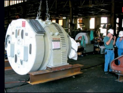
**MAIN ALTERNATOR** type AR10 with three phase companion alternator in one package, including rectifiers for traction power
